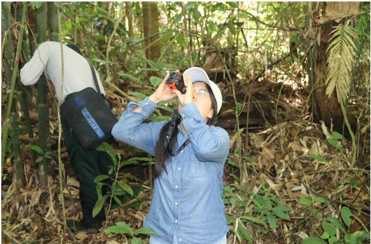
Measuring height of tree with tree' height measurement tool
